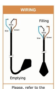
connection diagram enclosed to each float delivered.
